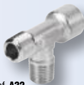
Ref. A32 Parallel male union tee with female side leg MMF
